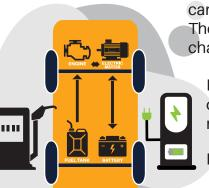
While HEVs can travel 1-2 miles before the gasoline engine turns on, PHEVs can go 10-40 miles before their gas engines need to provide assistance. They all are able to charge with a L2 charger, but most will not support fast charging.
